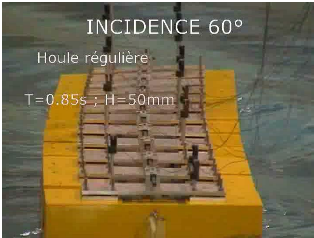
Segmented barge, experiments in BGO First, Toulon, France
