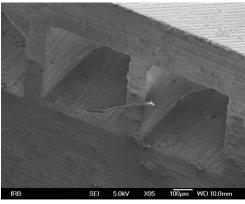
Fig. 2. Measured temperatures during fs laser operation with numerical simulation, left panel. SEM image of dental cavities formed by fs laser, right panel
