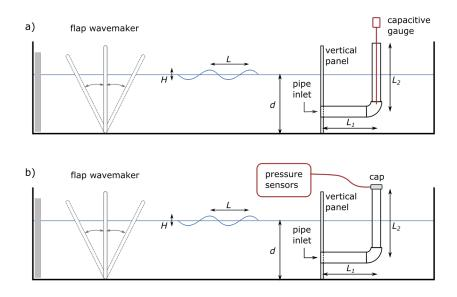
Figure 4: Scheme of the laboratory experiment for the open-end pipe case (A) and the closed pipe with a perforated cap case (B), not in scale
