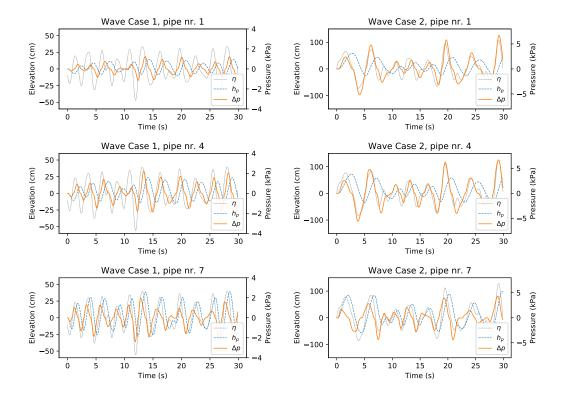
Figure 8: Comparison of sea surface elevations  $\eta$ , internal water level elevations  $h_p$  and air pressure drop  $\Delta p$  oscillations in pipes 1, 4 and 7, for wave cases 1 and 2 (30-sec excerpt)
