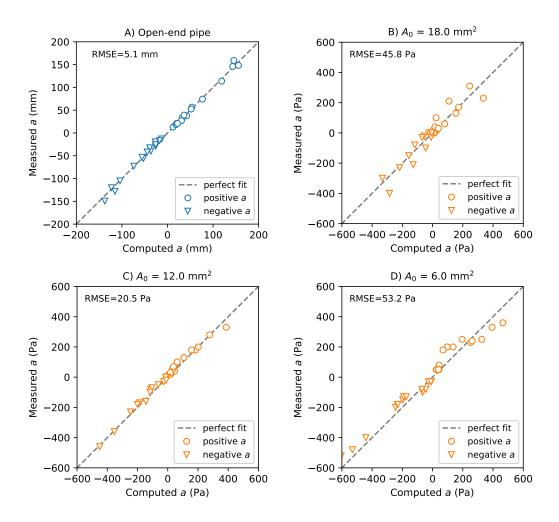
Figure 6: Comparison between measured and computed water level amplitudes for openend pipe (A) and air pressure amplitudes for closed pipes with orifice area  $A_0 = 18 \text{ mm}^2$ (B),  $A_0 = 12 \text{ mm}^2$  (C), and  $A_0 = 6 \text{ mm}^2$  (D)
