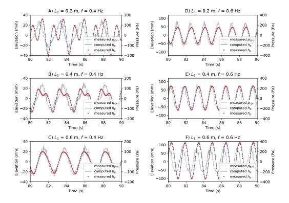
Figure 5: Comparison between measured and computed water level oscillations  $h_p$  for the open-end pipe and for different pipe lengths and wave frequencies (10-sec excerpt)
