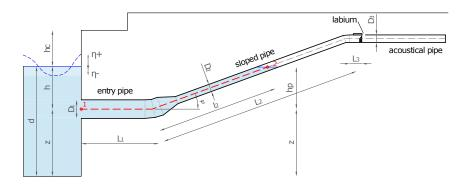
Figure 3: One-dimensional numerical model scheme of the organ pipe system
