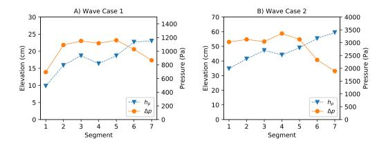
Figure 9: Mean amplitudes of water level elevation  $\eta$  and air pressure drop  $\Delta p$  in each segment of the Sea Organ for wave case 1 (A) and case 2 (B)
