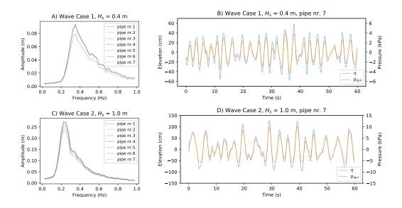
Figure 7: Generated wave amplitude spectrum and a 60-sec excerpt of water level  $\eta$  with corresponding dynamic wave pressure  $p_{wave}$  at the pipe inlet for wave cases 1 (A, B) and case 2 (C, D)
