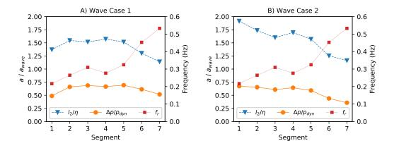
Figure 10: Mean amplitude ratio  $a/a_{wave}$  of the water level displacement  $l_2$  to sea surface elevation  $\eta$  and the ratio of the air pressure drop  $\Delta p$  to dynamic wave pressure  $p_{dyn}$  for wave case 1 (A) and case 2 (B), as well as corresponding resonance frequencies for each segment
