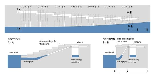
Figure 2: Plan and two characteristic cross sections of the Sea Organ in Zadar
