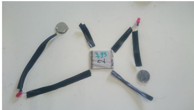
Figure 5: The detector variant with graphite lead on left hand side of the slab
