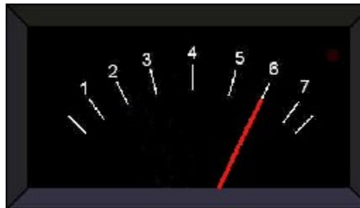
Slika 1.14 PPM (Peak Program Meter) metar.
