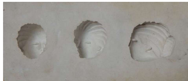
Figure 11. Molds made out of 3D model (courtesy of museum "Dom kulture Zvonimir" in Solin)
