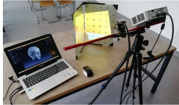
Figure 2. DAVID SLS-3 3D Scanner Slika 2. . DAVID SLS-3 3D skener
