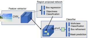
Fig. 2. The stages of Mask R-CNN
