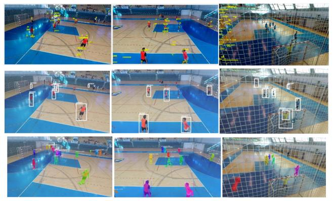
Fig. 6. MOG (upper row), YOLO (middle row) and Mask R-CNN (lower row) results on indoor sport footages
