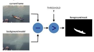
Fig. 4. The principle of background subtraction approach [15]
