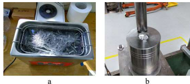
Figure 1. a) Chips cleaning utilizing ultrasonic bath b) Machined chips briquetting phase
