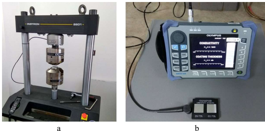
Figure 4. a) Universal tensile testing machine "Instron 8801" b) Eddy current measuring device
