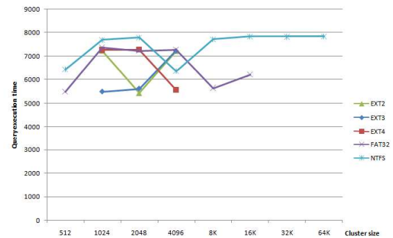
Figure 9. Read action (execution time according to different file systems with different cluster sizes)
