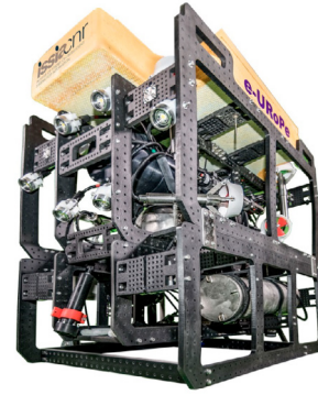
Fig. 2. e-URoPe hybrid AUV/ROV robotic platform used in the experiments.
