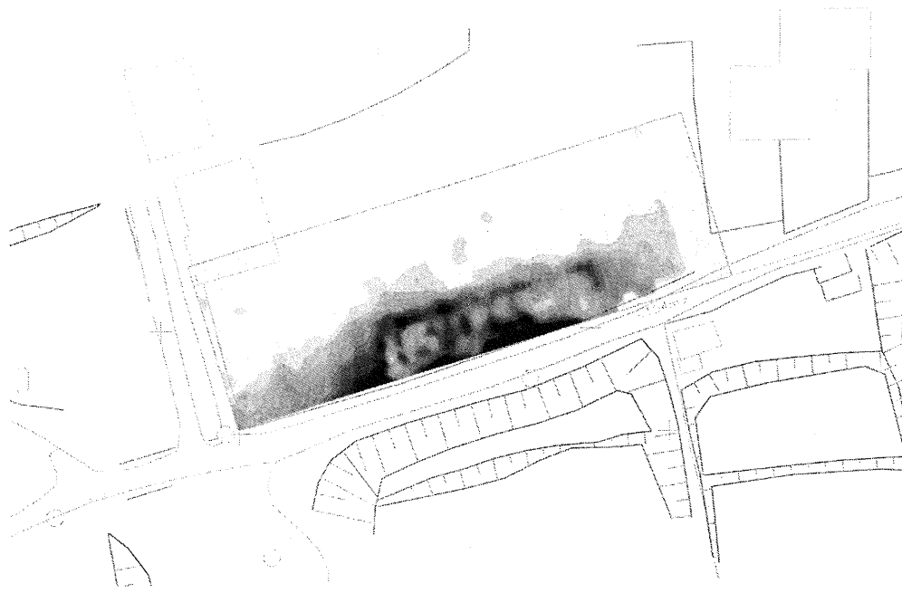
Fig. 2: Results of resistivity measurements on the direction of northern fortifications of Salona. High resistivity values represents efficiency of defence tower of rectangular shape.
