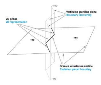
Figure 2. The concept of vertical boundary face strings
