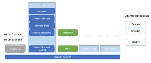
Figure 7 Technical components of DRDSI
