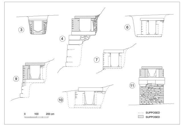
Figure 10. Different cross-sections of the channel (Authors)
