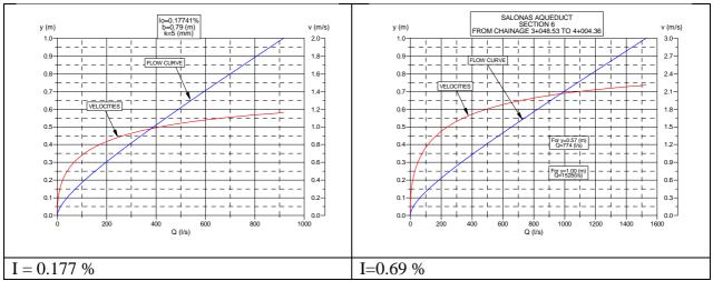
Figure 12. Flow curves of the channel at two typical sections with different bottom slope (Authors)
