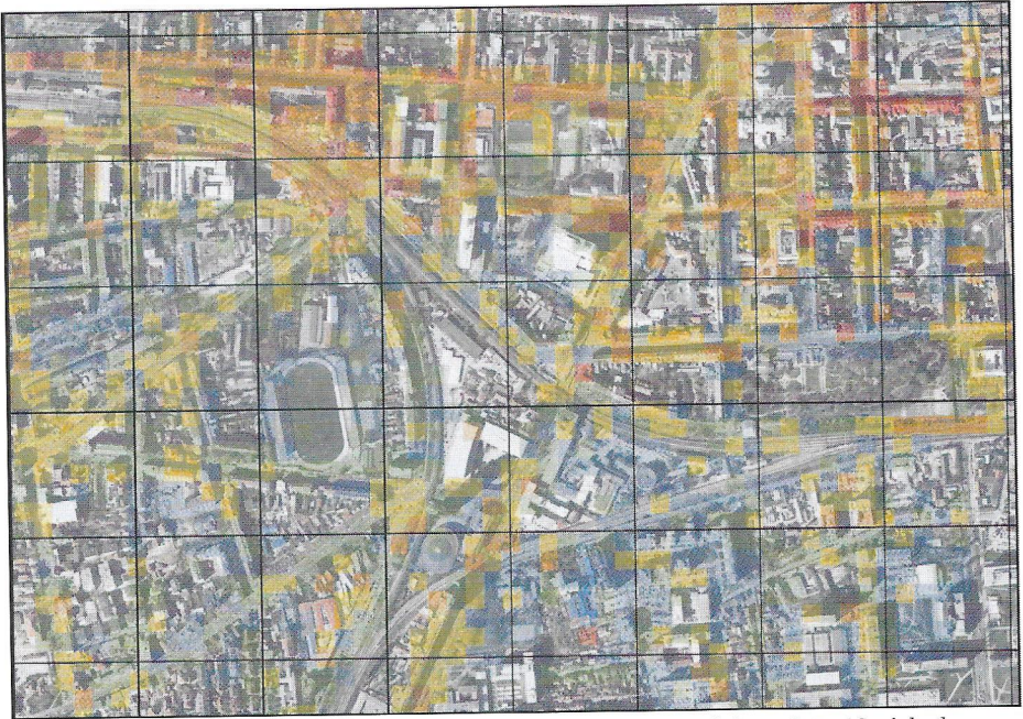
Figure 3.4 Noise map of a part of Zagreb for the period from 8 to 12 o'clock
