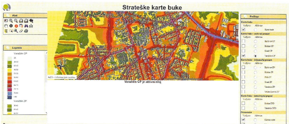
Figure 2.1 GIS Viewer of Strategic Noise Maps (The Strategic Noise Map of Varaždin) [URL 3]
