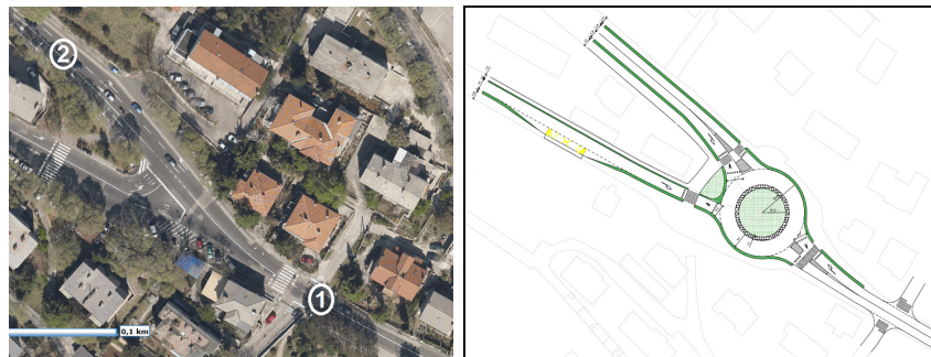
Figure 1. Present situation at intersection Case study 1 (left) and roundabout design at the same location (right) [13]
