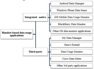
**Figure 3**: Classification and examples of smartphone data traffic monitoring applications
