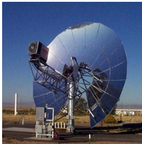
Figure 3.12 Stirling engine driven by solar heat [14].
