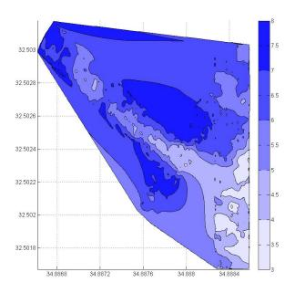
Fig. 7: Partial bathymetry map of the southern breakwater in Caesarea's outer harbor.
