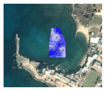
Fig. 6: Google Earth image of Caesarea's inner harbor with an overlaid bathymetry map.
