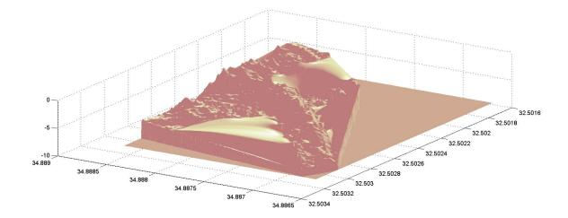
Fig. 9: Digital reconstruction of a 250 meters section of Herod's southern breakwater.
