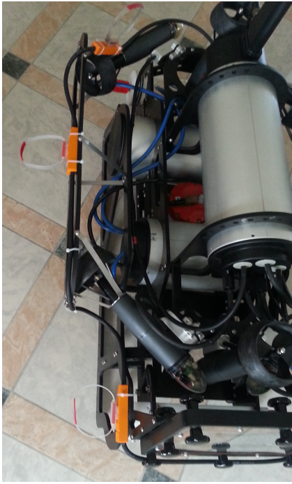
Figure 3. Kill switches installed on the vehicle
