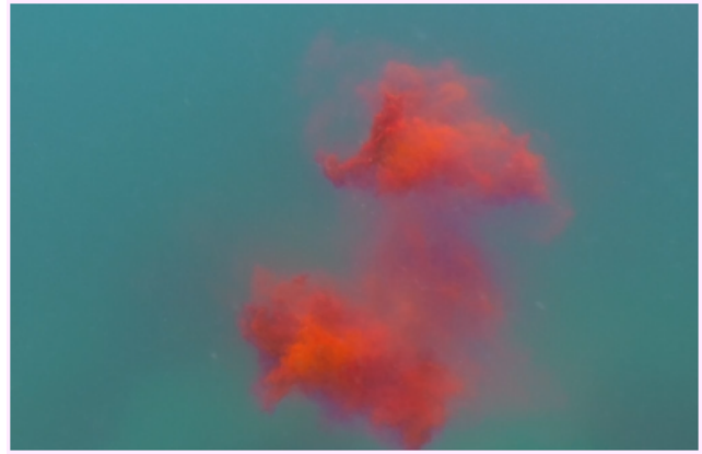
Fig. 4. Rhodamine plume, dispersed diluted tracer
