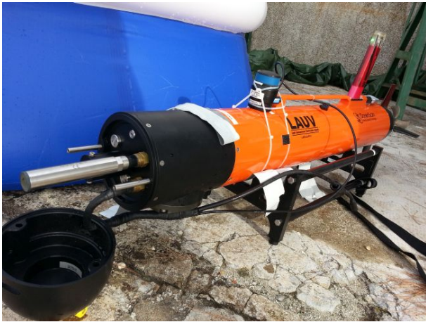
Fig. 1. LAUV AUV with removed nose section to present physical integration of the C7 sensor
