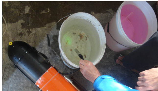
Fig. 5. Two point field calibration with 0 ppb and 100 ppb standards
