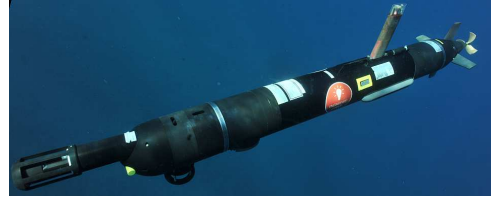
Fig. 2. AUV LAUV with Yellow fin side scan sonar in action
