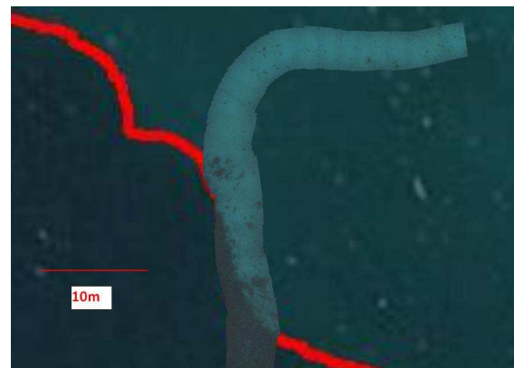
Fig. 5. Underwater Videomosaic overlaid over aerial image (white square in figure 4), used for upper depth limit detection
