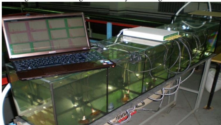
Fig.1. Optical cardiography system at one of the Moscow drinking water stations
