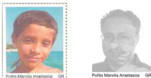
Picture 7. Printed sample of postage stamp with double portrait in visible(left) and infrared (right) spectrum.
