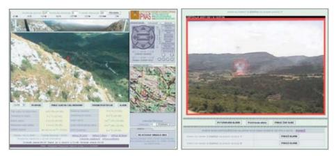
Figure 5 - iForestFire camera control screen with various manual control modes and typical fire alarm screen at location Buzet in Istria. The user can accept or discard the generated alarm.
