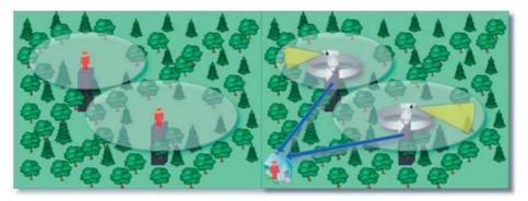
Figure 2 – The difference between human wildfire surveillance (left) and video camera based human wildfire surveillance (right)
