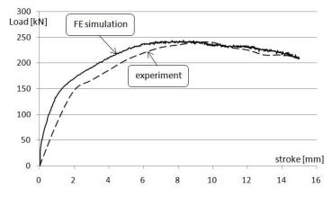
Fig. 7. Load stroke diagrams obtained by experimental investigation and FE simulation
