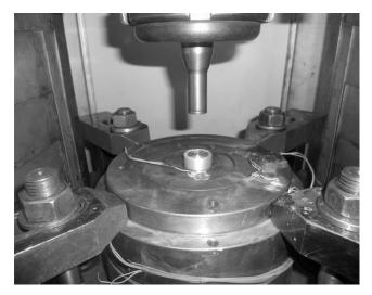
Fig. 4. Tooling for bi-metallic backward extrusion
