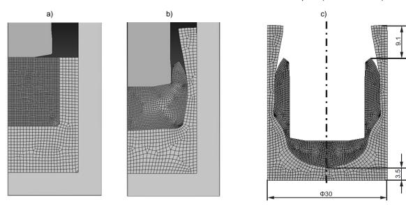
Fig. 6. Numerical simulation: a) start, b) intermediate phase after 6 mm punch stroke and c) end of the process (full cross-section)
