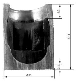
Fig. 5. Meridian cross section of the final experimental workpiece (stroke s = 15 mm)
