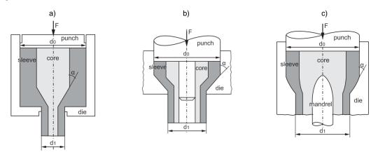
Fig. 1 Different variants of bi-metallic extrusion a.) forward extrusion b. and c.) tube extrusion
