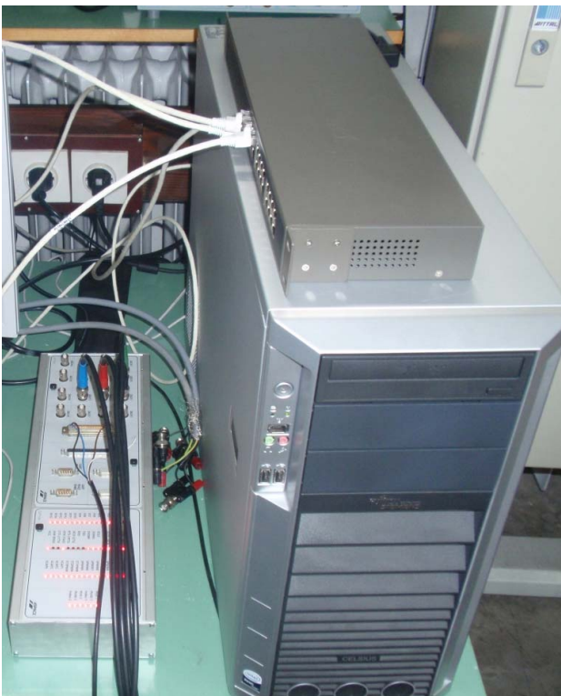
Figure 4. PC workstation with embedded dSPACE real-time controller board and its connector board
