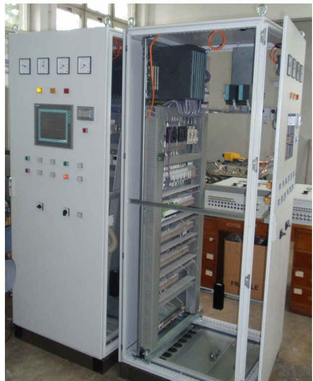
Figure 5. Turbine governor cubicles of HPP Lešće prepared for HIL testing
