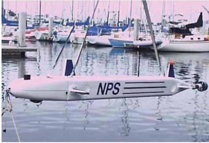
Fig. 9. The Aries , demonstrating the body-plan and general type of the model dynamics. Image from the public domain.
