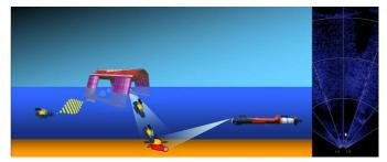
Figure 1. Mine reacquisition and neutralization: a highly capable SWATH ASV or hover-capable AUV guiding a low-cost expendable UUV to the sea mine (left); automated UUV (white dot) tracking from the sonar imagery (right).
