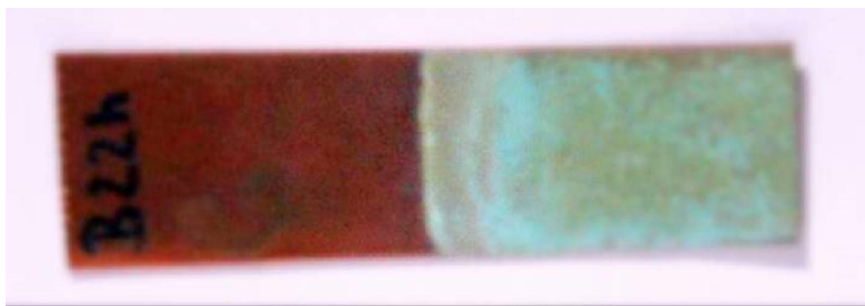
Figure 3.19: Bronze sample with the chloride patina formed by chemical – thermal procedure.
