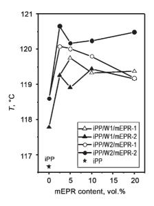
FIGURE 5 - Crystallization temperature ( $T_{\rm c}$ ) as a function of mEPR content<sup>24</sup>
