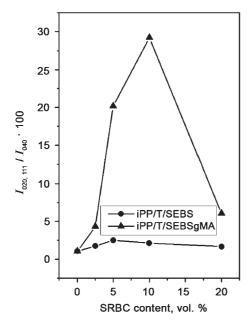
FIGURE 9 - Intensity ratio  $I_{020,111}/I_{004}$  of corresponding talc reflections in dependence on SRBC elastomer added to the iPP-1/T-3 88/12 composites<sup>26</sup>
