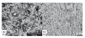
FIGURE 8 - Optical micrographs of (a) iPP-2/W-2/SEBS-g-MA (92/8  $\pm$  20) composite,  $^{23}$  and (b) iPP-2/W-2/mEPR2 (92/8  $\pm$  20) composite  $^{24}$
