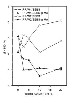
FIGURE 2 - B parameter (as a measure for  $\beta$ -iPP phase content) of iPP-2/W/SRBC composites as a function of SRBC content<sup>23</sup>
