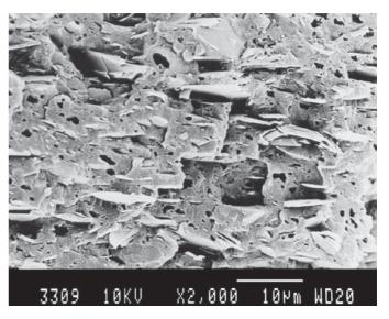
FIGURE 7 - SEM micrographs of xylene etched iPP-1/T-3/SEBS  $78/12/10 \text{ composite}^{26}$
