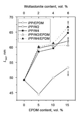
FIGURE 3  $L_{\rm 040}$  crystallite size of the iPP-1/W/EPDM composites in dependence of EPDM and wollastonite contents<sup>22</sup>
