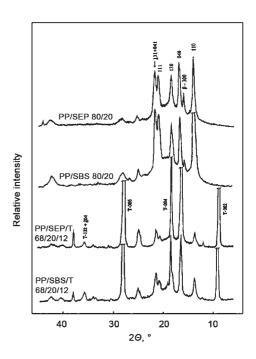
FIGURE 1 - WAXD diffractograms of the iPP-1/T-3/SRBC composites  $^{25}$
