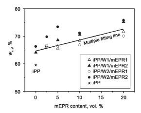
FIGURE 6 - Overall degree of crystallinity,  $W_{\rm c,x}$ , of composites recalculated on the iPP-2 polypropylene mass unit as a function of the mEPR content
