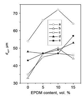
FIGURE 14 - Spherulite diameter as a function of elastomer content for (a) iPP/EPDM blend, and iPP/W-2/EPDM composites<sup>22</sup> with (b) 2 vol.% and (c) 4 vol.% of W2, as well as iPP/W-4/EPDM composites with (d) 2 vol.% and (e) 4 vol.% of W4
