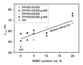
FIGURE 4 -  $L_{\rm 110}$  crystallite size of the iPP-1/W/SRBC composites in dependence of SRBC content<sup>23</sup>
