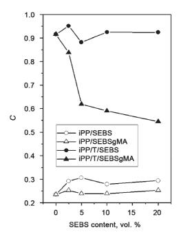
FIGURE 10 - Dependence of orientation parameter  $\it C$  of the iPP-1/SRBC blends and iPP-1/T-3/SRBC composites on elastomer content<sup>26</sup>
