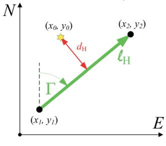
, as shown in Figure 1c). Now, the vertical distance is calculated as the distance of  $P_0$  to the line described with  $P_1$  and  $P_2$ , and is given with (6)
