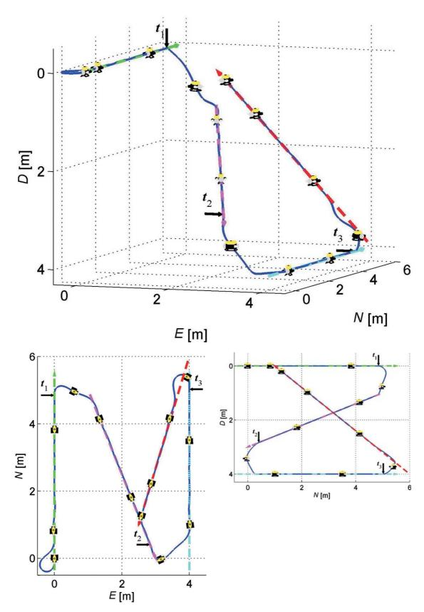
Figure 7 Path of the underwater vehicle in a) the NED frame, b) the N - E plane, and c) the N - D frame Slika 7 Putanja ronilice u a) NED koordinatnom sustavu, b) N - E ravnini i c) N - D ravnini
