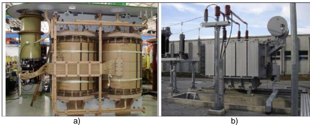
Figure 5 – a) Assembled active part of 16 MVA unit in the workshop and b) completed 15 MVA transformer at site during operation.
