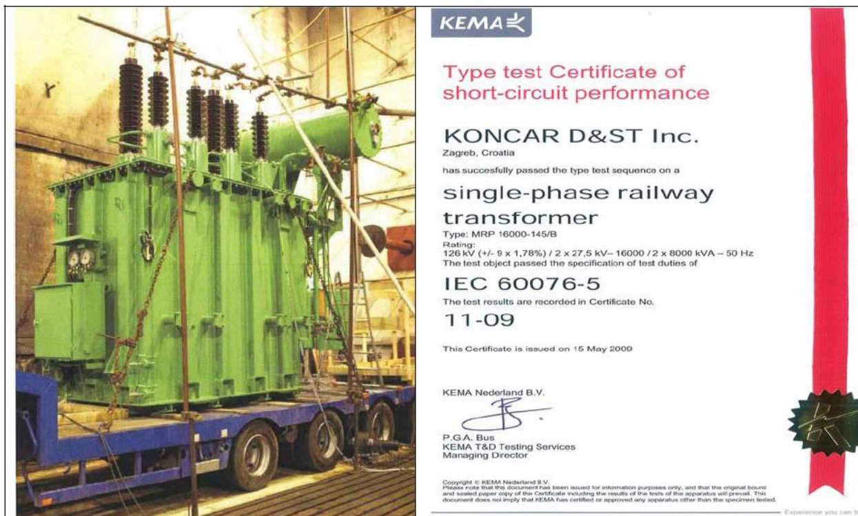
Figure 8 – a) Transformer during short-circuit withstand test in KEMA High Power Laboratory and b) Type test Certificate of short-circuit performance.
