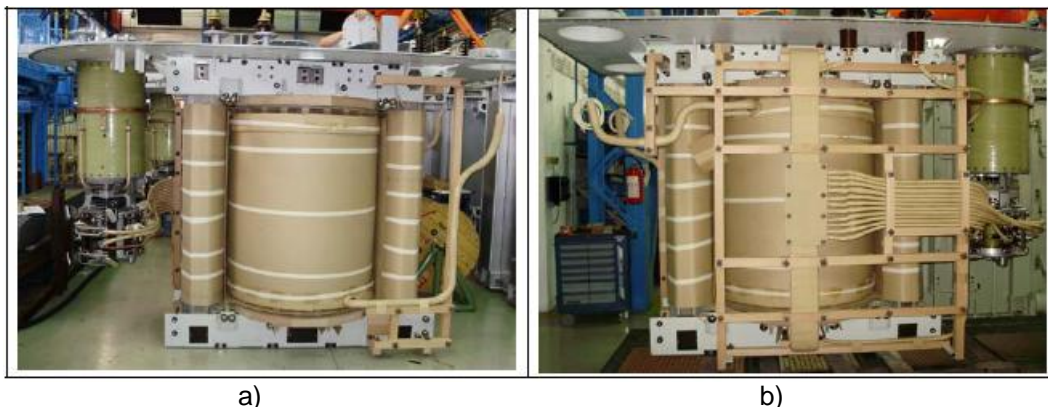
Figure 3 - Active part of 7.5 MVA traction transformer: a) HV terminal side, b) regulating winding connections to OLTC
