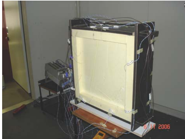
Figure 3. The test rig for prefabricated panel
