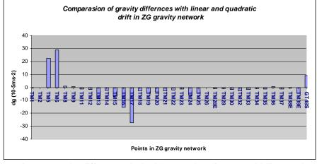
Figure 6. Gravity differences obtained between the adjustment with linear and the adjustment with quadratic drift in the Zagreb Gravity Network
