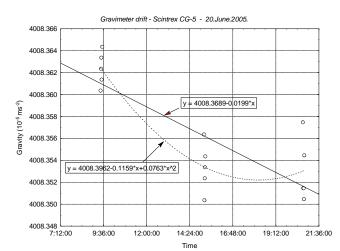
Figure 5. Linear and quadratic drift of the CG-5 gravimeter for the day 20.06.2005
