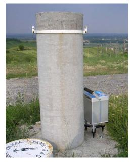
Figure 4. Typical GPS pilar of the Zagreb network
