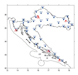
Figure 1. The 0. and I. Order Gravity Networks of the Republic of Croatia
