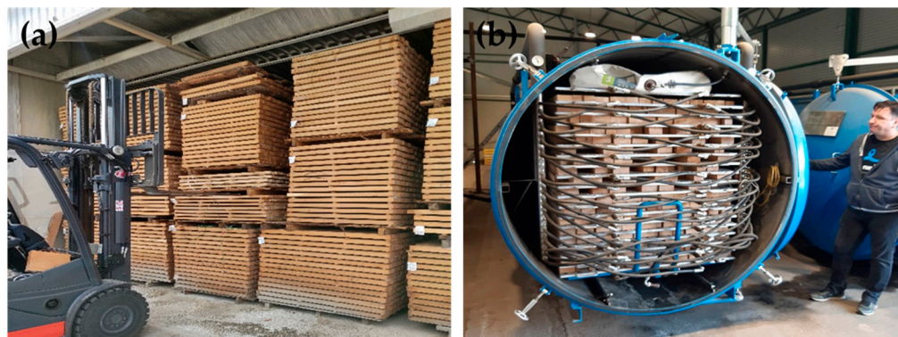
Figure 2. Normal temperature convection kiln drying (KD) of test oak samples (a) and vacuum drying (VD), using hot plate method for heat transfer (b).
