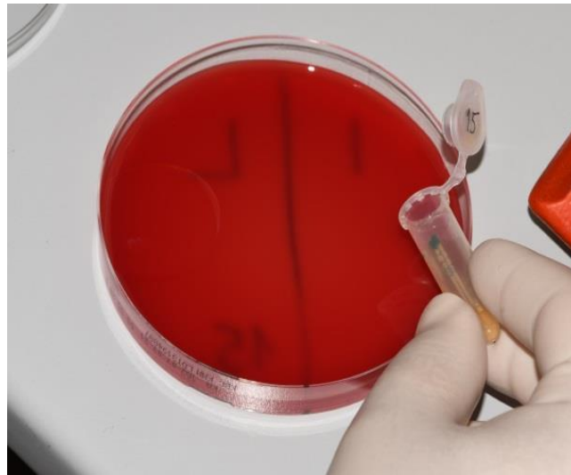
Figure 8. Application of the sample on to 5% blood agar.
