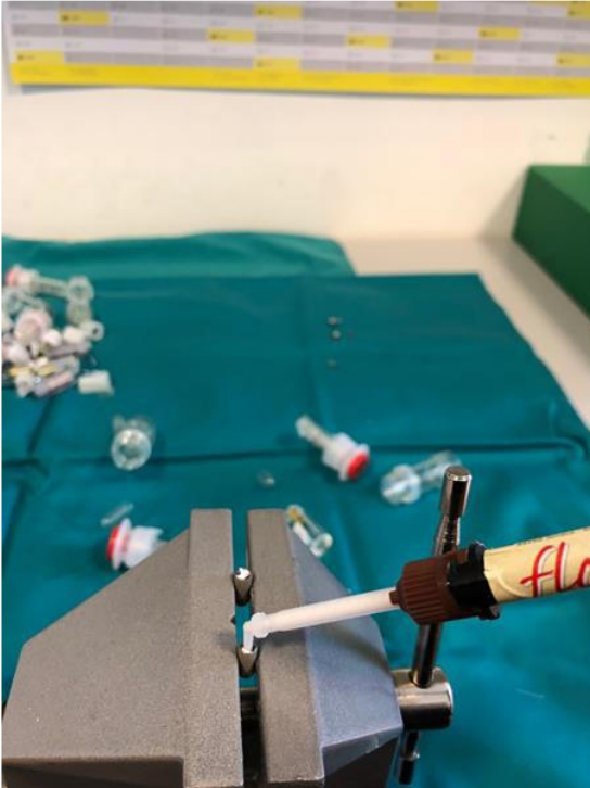
Figure 5. Flow.sil material application.
