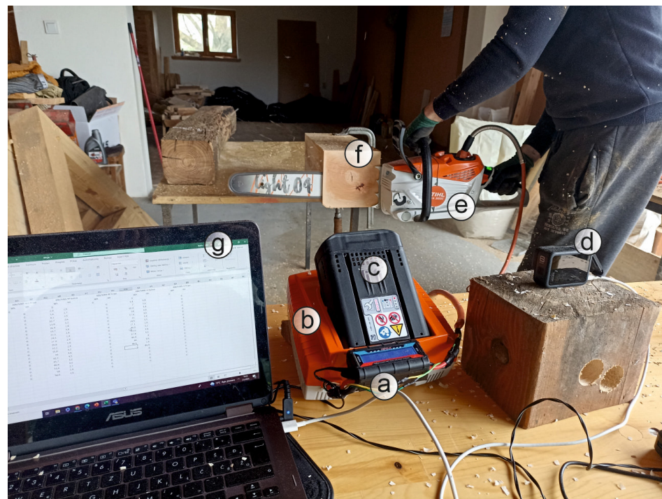
Figure 1. Measuring setup (a—multimeter Pichler C7282, b—Stihl AL300 charger housing, c—battery pack, d—GoPro ® camera, e—chainsaw, f—wood beam, g—field computer).
