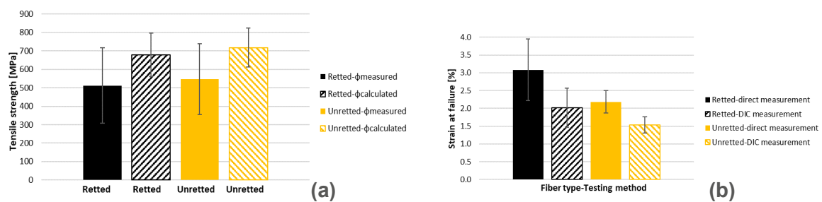
Fig.1 Single fiber tensile test results of retted and unretted fibers: (a) strength, (b) strain
