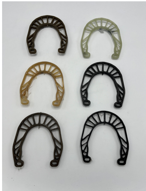
Figure 3 – Brake booster specimens of each material: hemp, E-glass, viscose, basalt, flax, and carbon (from top to bottom - left to right).
