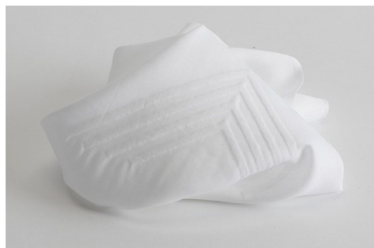
Fig.1 Textile screen print with Screen print with 4.2mm line thickness generates a strong puffed surface effect on the fabric with light pleats at the end of the print line.
