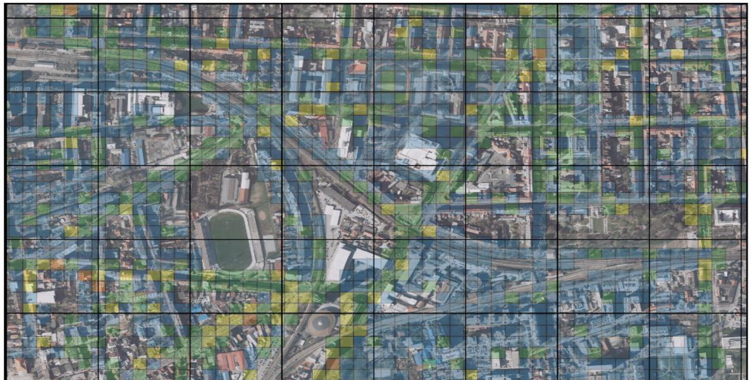
Noise map of the part of the city of Zagreb for the period from 18:00 to 22:00
