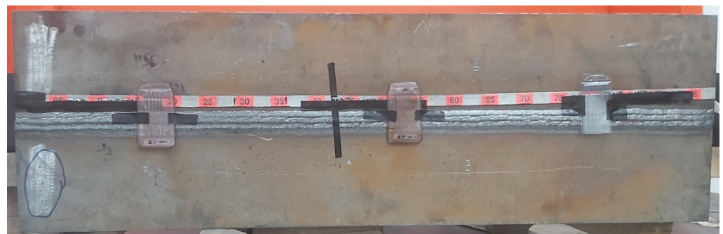
Figure 2. X-welded joint radiographic testing (RT) according to ISO 17636-1.
