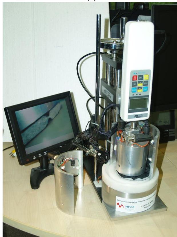
Figure 3. Multi-purpose differential conductometer: (a) schematic diagrams; (b) realized device.
