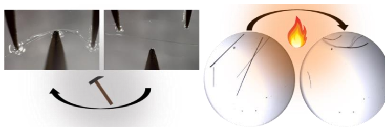
Figure 1. Mechanically and thermally compliant single crystals of copper(II) coordination polymer.
