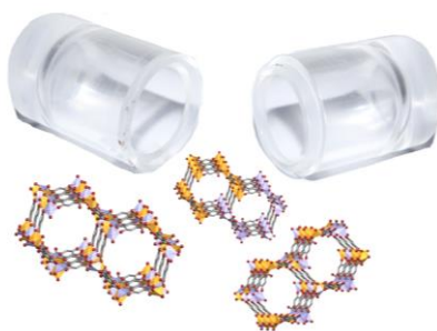
Figure 1. Magnetic Cu-Zn MOF-74 materials synthesized by mechanochemistry.
