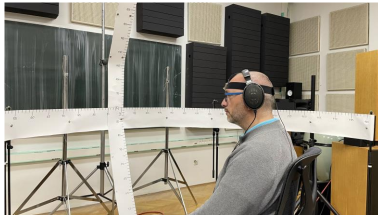
Figure 3. A participant with head-mounted binaural system elements on a rotating chair, tracking the virtual sound stimulus.
