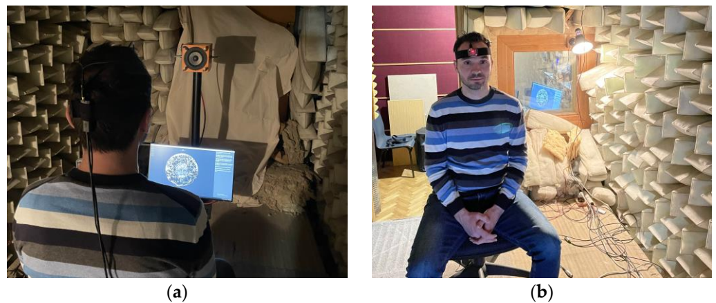
Figure 1. HRTF measurement in the anechoic chamber: (a) back view of a participant; (b) front view of a participant.
