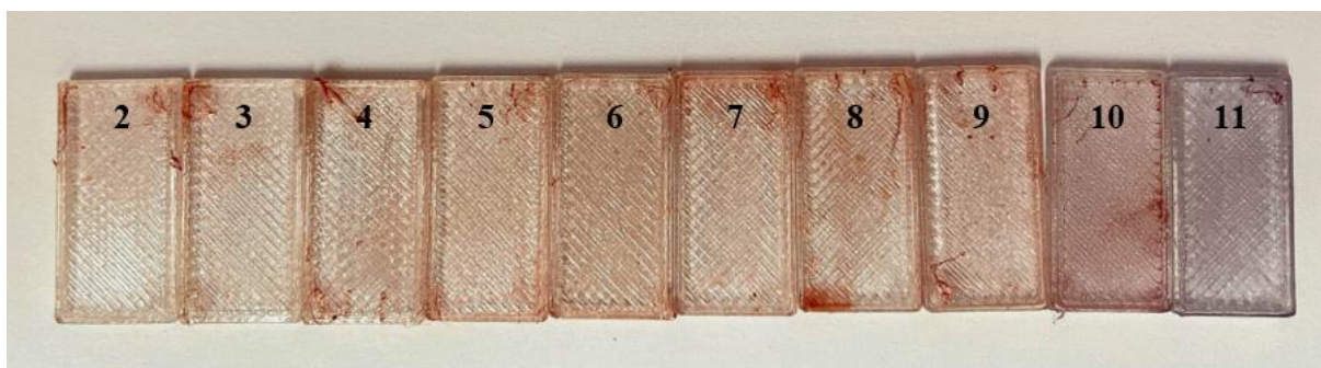
Fig. 1: Test plates with litmus-based sensor films after 10 minutes in pH solutions.
