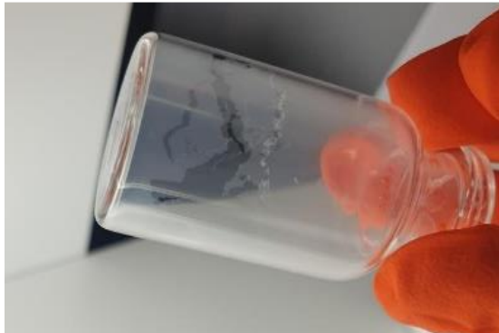
Fig. 1: Glass vial 10R, colorless, tubular glass, hydrolytic group I, after 3 hours autoclave treatment on 121 °C filled with 0.1 M KOH.
