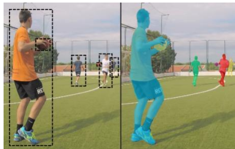
Fig. 1 Marking objects with a bounding box (left) and object segmentation marking pixels belonging to an individual object (right) (Burić et al. 2020)
