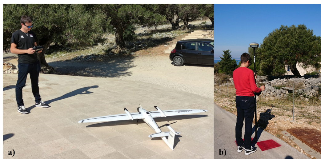
Figure 3. Field work; (a) Trinity F90+ MS mission; (b) Trimble R8s CPs and RP collecting.
