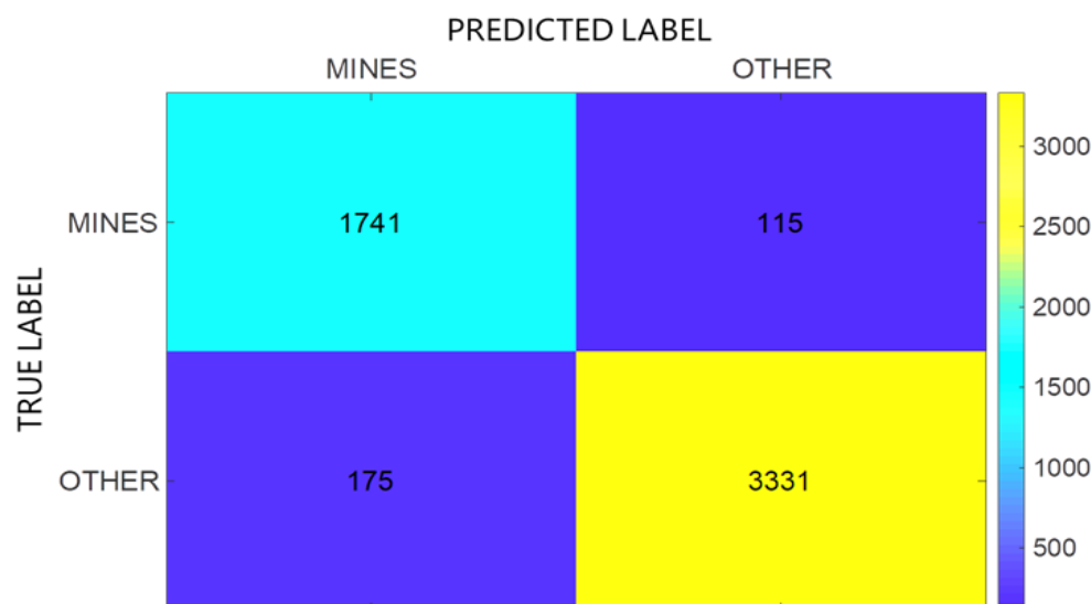
Figure 12. Confusion matrix of the detection algorithm for the Vegetation Monitoring Device (VMD).
