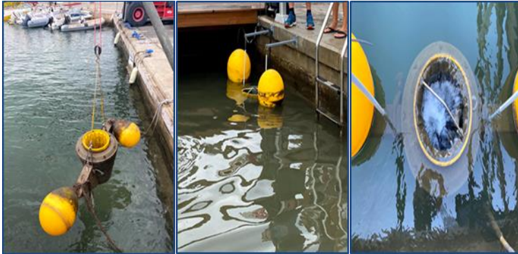
Figure 4: Seabin device installed in Port of Cristo and Port of Colonia de Sant Jordi.
