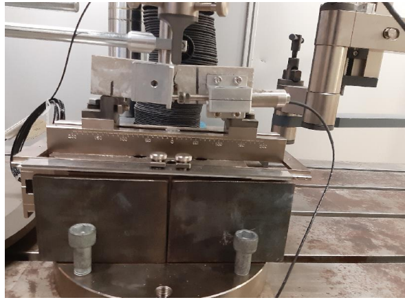
Fig. 1. Experimental setup for the three-point bending test.
